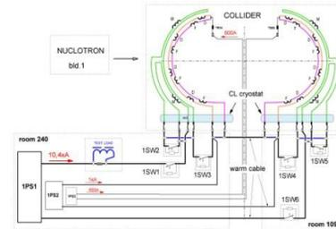
Figure 9: The basic wiring diagram of the power supply of the 1st ring of the Collider. The blue color shows the equivalent load and its connection circuits.
