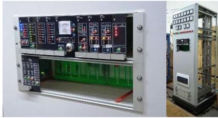
Figure 6: Control racks with a crate of the electronics of the Nuclotron power system.
