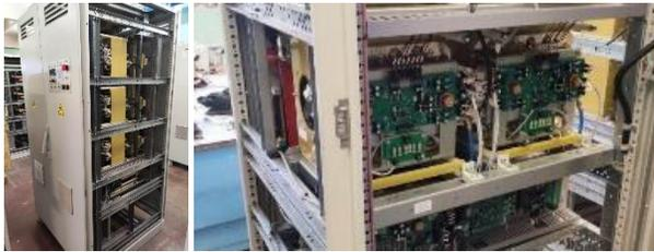
Figure 3: PIT11-50, general view of the PWM converter cabinet and the PWM converter power module.
