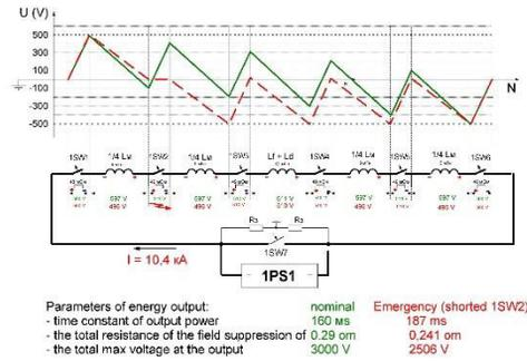
Figure 4: Plot of the potential of the structural magnets during evacuation of 10.4kA current: the normal mode is the green solid line, the emergency mode due to a defect of SW2 is the red dotted line.
