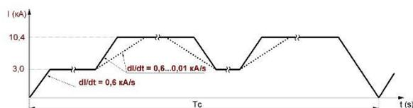
Figure 1: Current cycle of Collider magnets.
