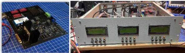
Figure 7: CMC measuring card and the view of the CMC unit.
