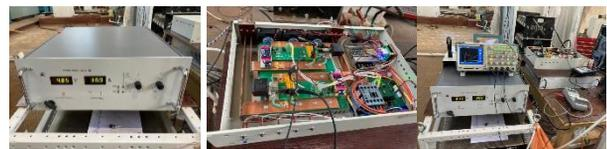
Figure 5: Testing a source with an EED (from right to left SM 15-400, EED300-70, and test bench).
