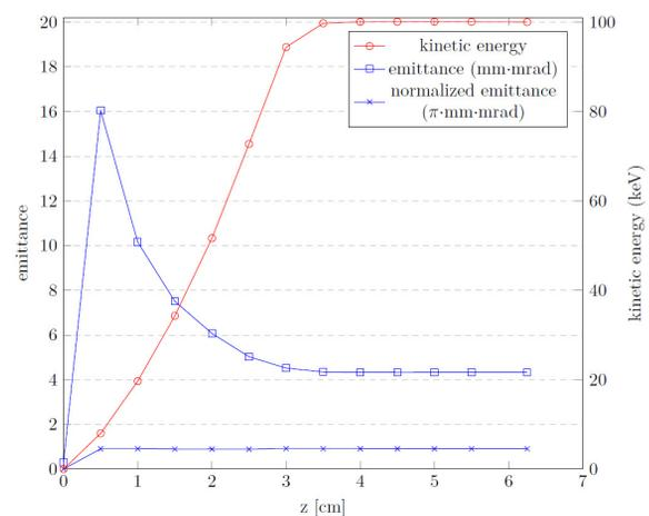
Figure 4: The emittance and kinetic energy of the electron gun along the beam trajectory.
