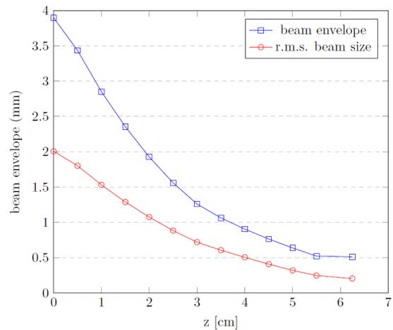
Figure 5: The beam envelope and rms beam size along the beam trajectory.
