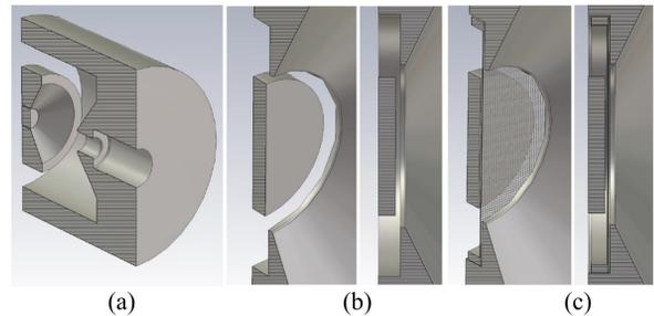
Figure 1: The model of electron gun in CST with (a) a complete model, (b) a gun-without-grid model, and (c) a gun-with-grid model.
