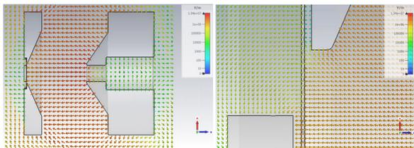
Figure 2: The electric field of the electron gun. The field near the cathode, grid and focusing electrode is shown on the right.
