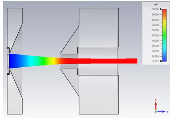
Figure 3: The electron beam trajectory of the electron gun.
