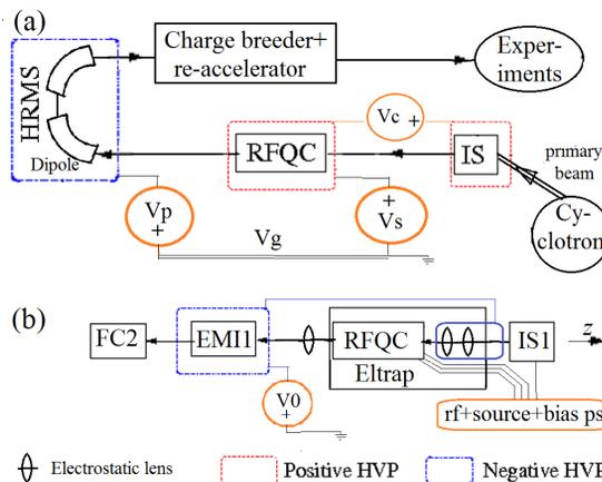
Figure 1: Block diagrams (not to scale) of: (a) interdependence of ion source IS, cooler and HRMS, as a zoom in the SPES project; (b) ion source IS1, cooler and emittance meter EMI1 in the Eltrap machine; beam stops at Faraday cup FC2. Some power supplies (ps) are sketched.
