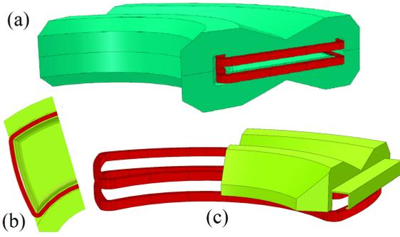
Figure 3: Optimization steps of dipoles with large bending radius (1.5 m): (a) from H-shape to yoke weight reduction; (b) adding Rogowsky edge with curved boundary (radius  $R_e \cong 2$  m to 3 m) of pole shoes; (c) view of coils, a field external clamp and a final chamfer of yoke.
