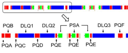
Figure 1: location of the magnetic element in the H6B cell: quadrupoles (red), sextupoles (green), dipoles (blue).
