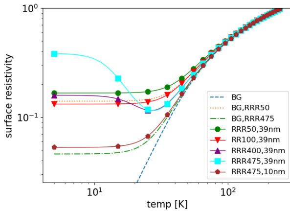
Figure 3: Comparison between calculations of new thin film surface resistivity theory with calculations using Reuter & Sondheimer with Bloch-Gruneisen resistivity. Note the minimum which appears for high purity, RRR, copper.
