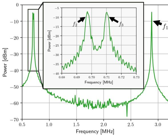
Figure 3: Exemplary excitation spectrum for the slow extraction of a carbon-ion beam with  $E_{\text{kin}} = 124.25$  MeV/u. The three frequencies correspond to fractional tune values of  $q_0 = 0.679$  and  $q_1 = 0.673$ , where both  $q$ -values are excited at the lower first harmonic and  $q_1$  is also excited at the lower second harmonic.
