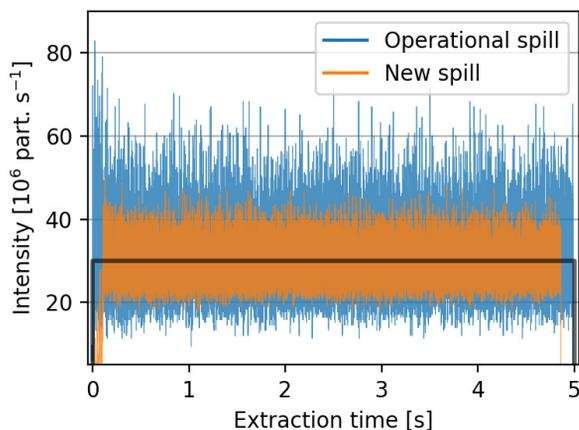
Figure 6: IC measurement of spills at 20 kHz with a carbon-ion beam  $C^{6+}$  with  $E_{kin} = 316.92$  MeV/u. Blue: Operational spill recorded with the nominal scheme for extraction. Orange: Spill recorded with the described signal.
