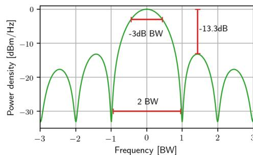
Figure 2: The symmetrical base band BPSK spectrum generated with a PRN has a -3 dB-bandwidth of  $BW = f_{PRN, clock}$ , the zeros of the spectrum are at  $n \cdot BW$  and the first side band is suppressed by -13.3 dB.
