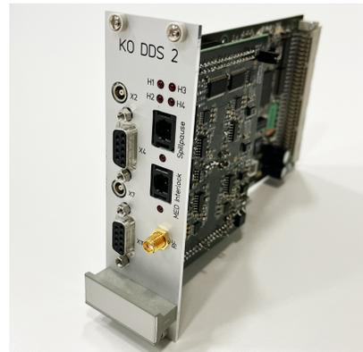
Figure 5: The new KO DDS 2 consists of a FPGA based motherboard and a RF daughter board. It also includes the interlock system for spill pause and spill abort features.
