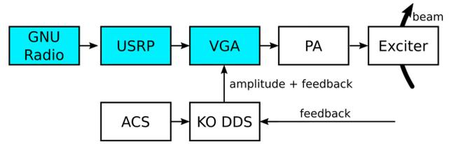
Figure 4: Block diagram of the experimental setup: The USRP generates the spectrum described above which is modulated by the variable gain amplifier (VGA) with the amplitude set value from the data supply model and the correction feedback loop provided by the ACS over the KO DDS. The LLRF signal is amplified by the PA and fed to the exciter.
