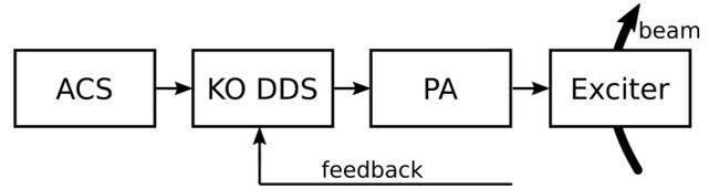
Figure 1: RF KO setup from the ACS, the Direct Digital Synthesizer (KO DDS), the power amplifier (PA) to the exciter, including the feedback for the intensity loop.
