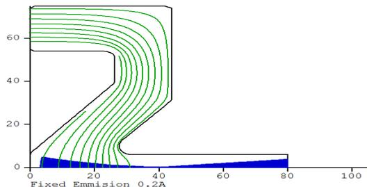
Figure 2: 200mA beam simulation results in EGUN.
