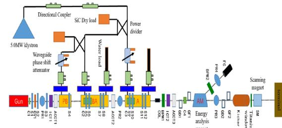
Figure 1: Layout of 10 MeV electron accelerator.
