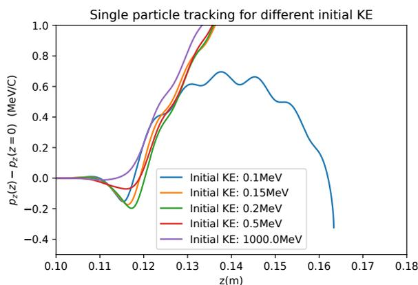
Figure 3: Trajectory of single particles for different initial energies.
