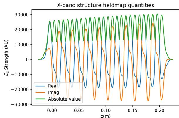
Figure 1: X-band structure fieldmap used.
