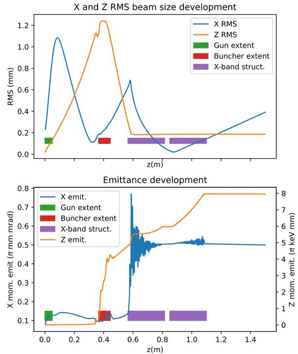
Figure 6: Development of bunch RMS and emittance through beamline.
