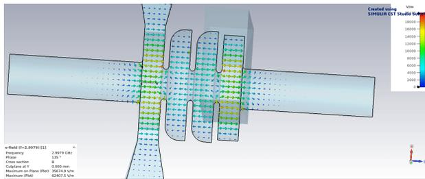
Figure 5: 3D model of buncher.
