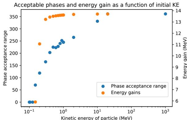
Figure 2: Acceptable for transmission phase range, and maximum energy gain for a given initial kinetic energy.
