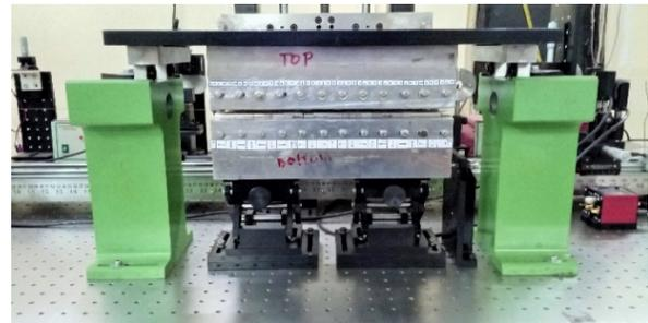
Figure 9: 300 mm length asymmetric undulator.
