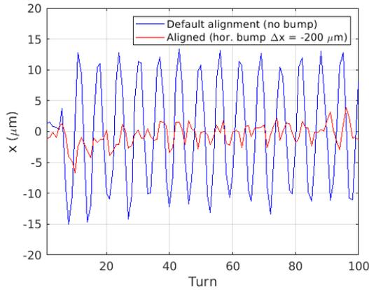
Figure 2: By default the stored beam is not perfectly aligned with the magnetic center of the MIK which results in betatron oscillations when the MIK is triggered (blue). The perturbation is minimized when the beam is centered thanks to a horizontal bump of  $-200\ \mu\text{m}$  (red). Both signals are averaged over 10 acquisitions.
