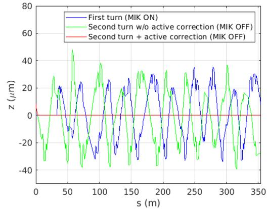
Figure 1: Vertical COD due to the residual dipolar error. The MIK perturbs the beam which exhibits large betatron oscillations during the 1<sup>st</sup> (blue) and 2<sup>nd</sup> (green) turns without correction, for  $\nu_z = 0.339$ . The amplitude of the residual betatron oscillations is canceled when the corrector is switched on during the 2<sup>nd</sup> turn (red).
