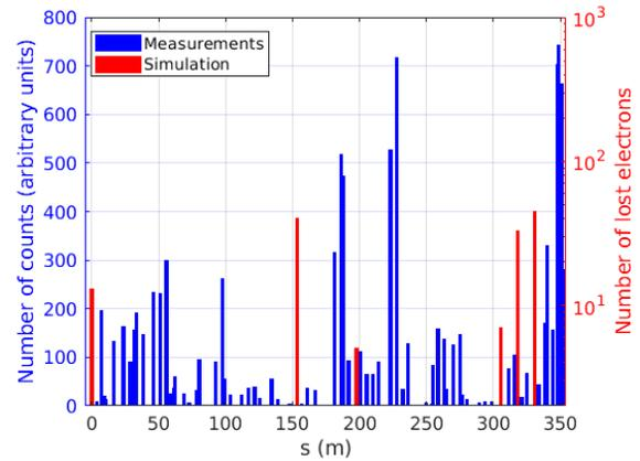
Figure 3: Injection loss map along the ring. The BLM signals (blue bars) give the number of counts, averaged over the first 200 turns in the ring, due to particle showers ignited by electron losses. The simulation (tracking of a Gaussian bunch beam of  $10^4$  electrons, at 10% coupling) gives the total number of lost electrons over the first 200 turns and their location in the ring (red bars).
