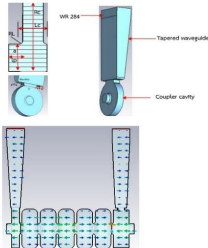
Figure 5: Coupling geometry and longitudinal electric field distribution of the 7-cells.
