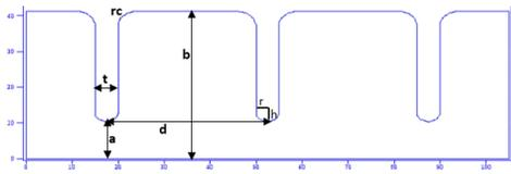
Figure 2: Schematic of three cells of TW electron linac.
