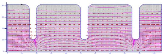
Figure 3: Electric field of the TM<sub>010</sub>- $2\pi/3$  accelerating mode.
