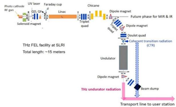
Figure 1: Layout of THz FEL source with the total length of 15 meters.
