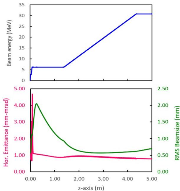
Figure 6: (top) Beam energy along z-axis and (bottom) Normalised transverse emittance (pink) and beam size (green) with 1 nC bunch charge.
