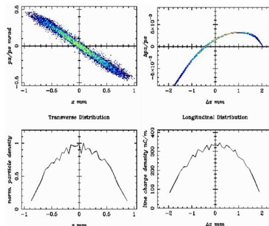
Figure 7: Phase space at the end of linac.
