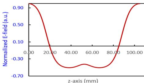
Figure 4: Electric field generated from three cells of TW electron linac.
