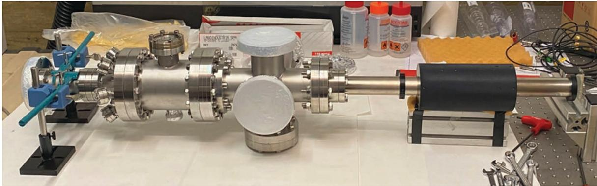
Figure 4: TRAMM vacuum system pre-assembled to check its functionality. We will start shortly the final installation and, afterwards, the apparatus commissioning.
