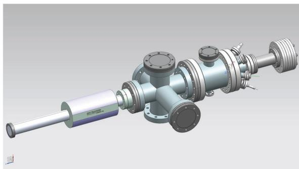
Figure 2: 3D model of TRAMM designed to be connectable to our preparation system. On the left the short UHV manipulator, in the middle the transport chamber and on the right the core of TRAMM, i.e. the detection system.
