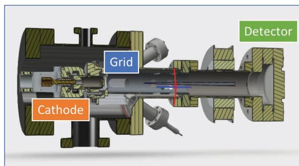
Figure 3: TRAMM detector inner view. Main components are the INFN plug where the photocathode is deposited, the grid accelerating system and the detector to convert the electron signal to an optical image.
