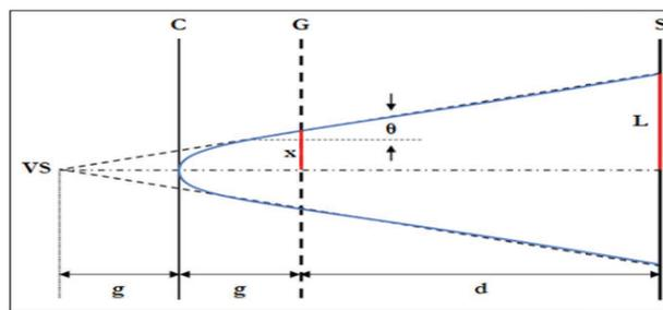
Figure 1: Schematics of the TRAMM experiment. Photocathode is placed at position C, grid in G and the screen at S.
