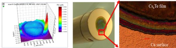
Figure 4: QE mapping of Cs<sub>2</sub>Te #2020.03.04 after three months operation (left). The photograph of this used cathode already exposed in air (middle). The film border under microscope (right).
