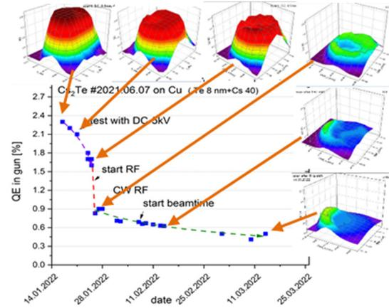
Figure 2: QE tracking of  $\text{Cs}_2\text{Te}$  #2021.06.07 with the QE mappings in different stages during operation in SRF gun.
