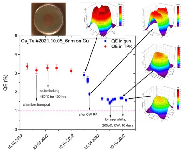
Figure 1: QE tracking of  $\text{Cs}_2\text{Te}$  #2021.10.05 before and after inserting into SRF gun. The red points are the QE measured in the transport chamber and the blue ones are those during SRF gun operation. The photograph of the cathode and the QE mappings in different stages are shown here as additional information.
