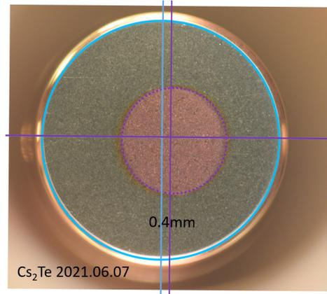
Figure 3: Photograph of the  $\text{Cs}_2\text{Te}$  cathode #2021.06.07 with 8 nm Te and 40 nm Cs, but 0.4 mm off centre.
