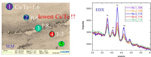
Figure 5: The SEM photograph of the film border of Cs<sub>2</sub>Te #2020.03.04 with the local Cs/Te ratio (left). The EDX spectra taken at the different location for Cs/Te ratio calculation (right).
