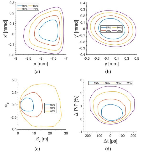
Figure 3: Contour indicating the expected efficiency of single-bunch aperture sharing injection into the Diamond-II storage ring for various mis-steerings and mis-match at the exit of the thin septum magnet.
