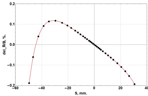
Figure 6: Good field region for the designed dipole magnet.  $S$  – line in horizontal plane through the center of the dipole magnet perpendicularly to the beam trajectory.  $0$  – position of the beamline center.
