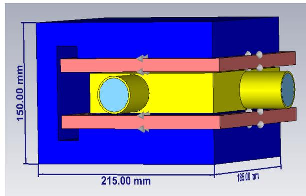
Figure 5: CST model of bending magnet.
