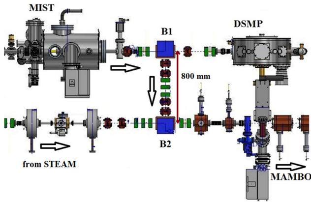
Figure 1: Scheme of the designed separation beamline. 90° dipole magnets (blue), quadrupoles (green), dipole correctors (brown). (By courtesy of Dr. Simon Friederich).
