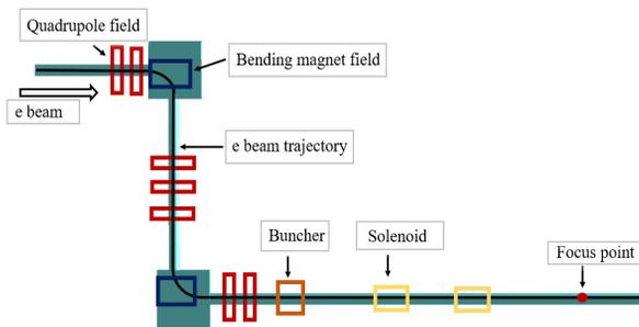
Figure 7: CST model of the injection beamline.  $90^\circ$  dipole magnets (blue), quadrupoles (red), solenoids (yellow), buncher (brown).
