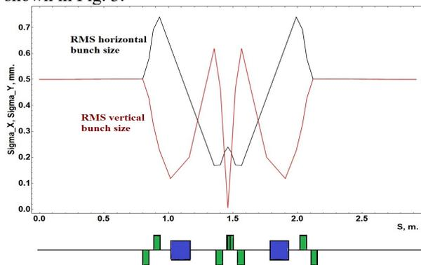
Figure 2: RMS transverse beam sizes in the separation beamline divergence and non-divergence plane.
