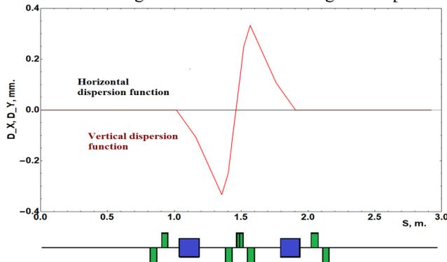
Figure 3: RMS dispersion functions in the separation beamline for the dispersive and non-dispersive plane.
