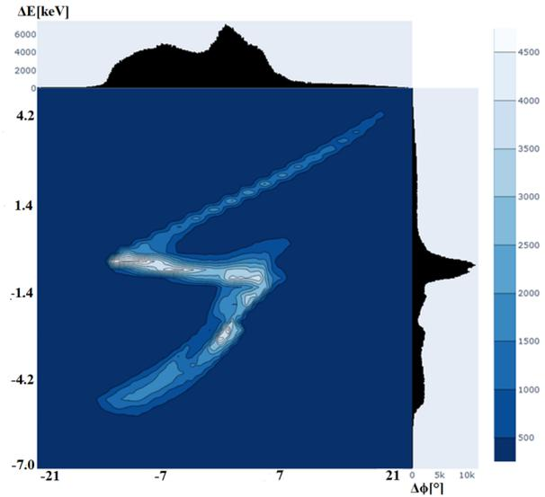
Figure 8: The longitudinal phase-space of the electron bunch in the entrance of the first acceleration section of MAMBO.
