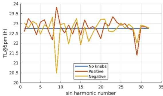
Figure 4: Effect of the sine wave octupolar knobs on the Touschek lifetime.
