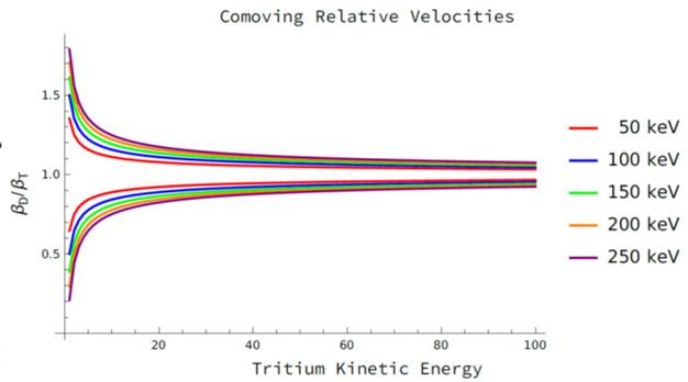
Figure 2: The relative velocity of the deuterium compared to the tritium for a variety of tritium energies and center of mass energies
