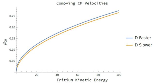
Figure 3: This is the center of mass velocity for the D-T system at 65 keV center of mass energy, which has the highest cross section
