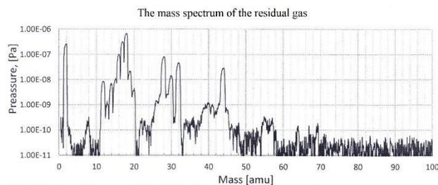
Figure 2: Total mass spectrum of residual gases at the end of the vacuum tests.
