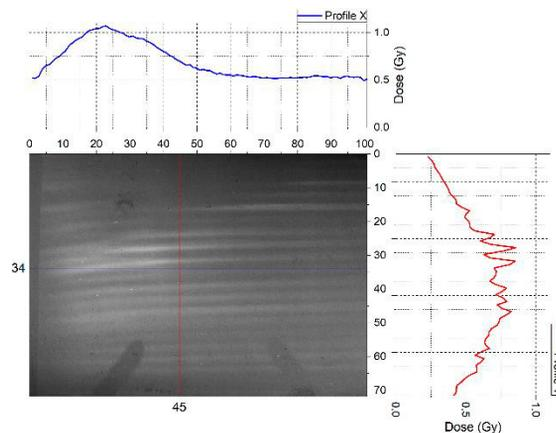
Figure 8:  $^{12}\text{C}^{4+}$  ion beam spot on the monochrome film.
