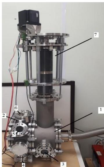
Figure 6: External view of vacuum chamber 1 and 2 with the positioning system and the stepper motor.
