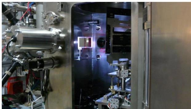
Figure 5: Internal view of the SOCHI vacuum chamber.
