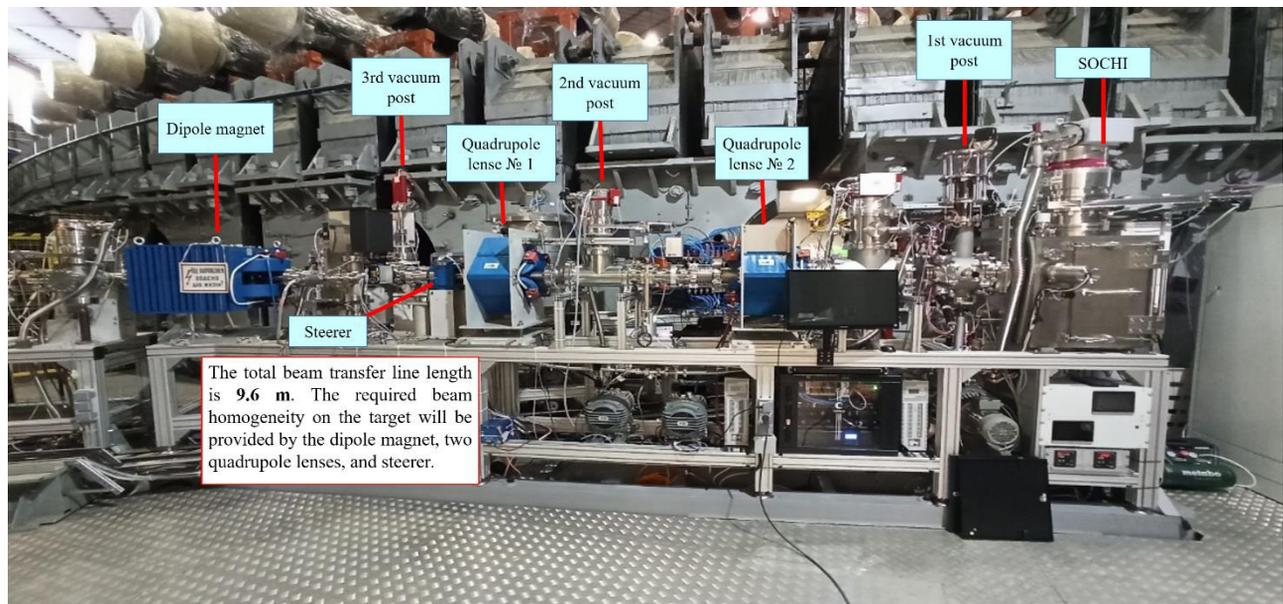
Figure 3: SOCHI beam transfer line and the applied station.
