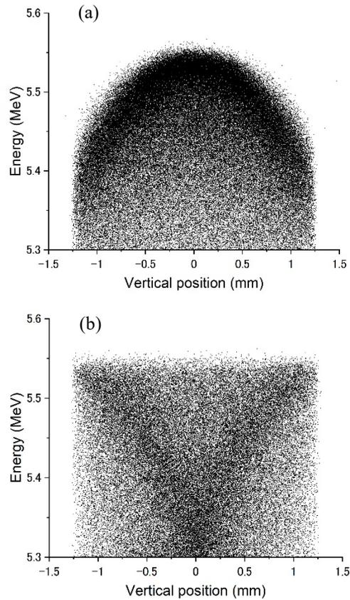
Figure 3: LCS gamma-ray energy distribution in the vertical axis with the undulator  $K$ -value of (a)  $K=0$  and (b)  $K=0.2$ .
