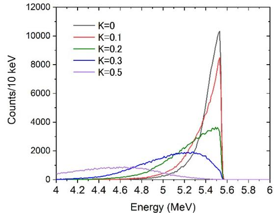
Figure 4: Energy spectra of the gamma-ray beams with different  $K$ -values from 0 to 0.5.
