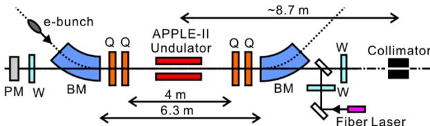
Figure 2: Schematic drawing of the BL1U beamline in UVSOR. Optical Klystron type undulator containing twin helical undulators of APPLE-II type and a buncher magnet are installed in 4.3 m free space. PM: power meter, W: window, SM: Spherical Mirror.
