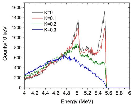
Figure 6: LCS energy spectra calculated EGS5 including Ge detector response.
