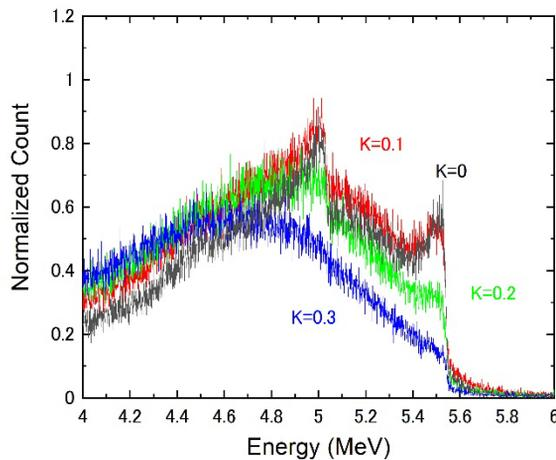
Figure 5: Measured LCS beam spectra with the undulator K-value of 0, 0.1, 0.2, and 0.3. The LCS beam was collimated with 2 mmφ lead collimator.
