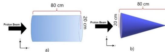
Figure 1: Fixed cylindrical and conical spallation target.
