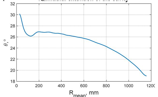
Figure 6: Azimuthal extension of the cavity (between middles of accelerating gaps).
