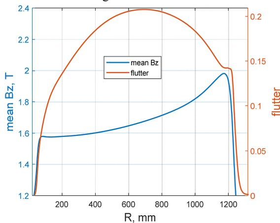
Figure 3: Average magnetic field and flutter along the radius.
