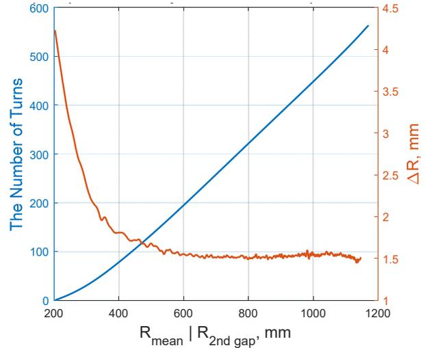
Figure 9: Number of turns (blue dashed line) and orbit separation distance (red solid line) in the cyclotron along the radius.
