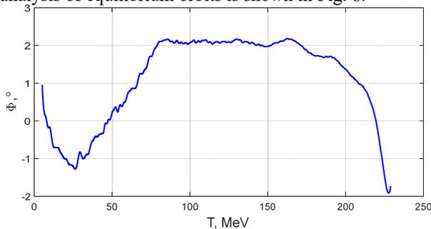
Figure 8: Integral phase shift along the radius. Positive phase corresponds to the lagging particle
