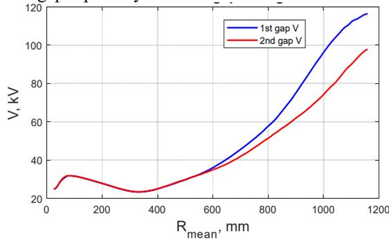
Figure 7: Accelerating voltage along radius.
