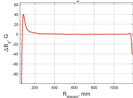
Figure 4: Difference between average and isochronous field.
