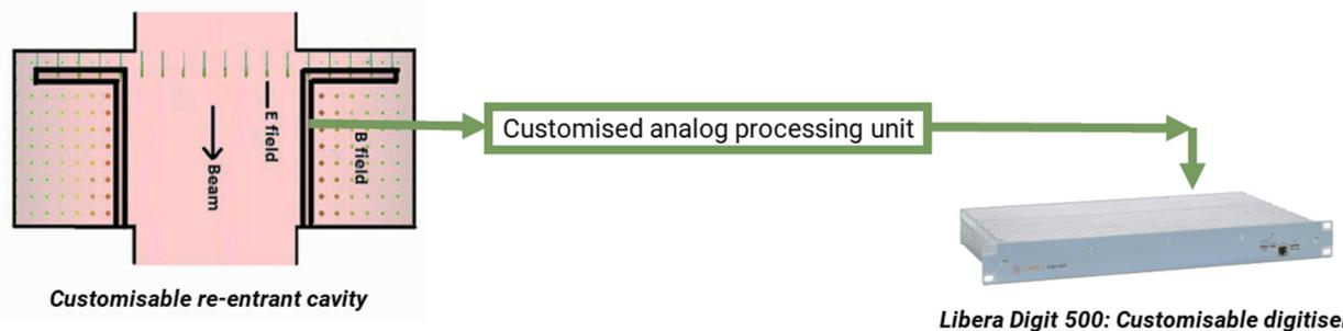
Figure 3: Graphical representation of the non-interceptive turn-key diagnostic system, CRCDS (Cavity Resonator Current Diagnostic System). The re-entrant cavity and the analog processing unit to be developed by Bergoz Instrumentation and the digital solution developed by Instrumentation Technologies.
