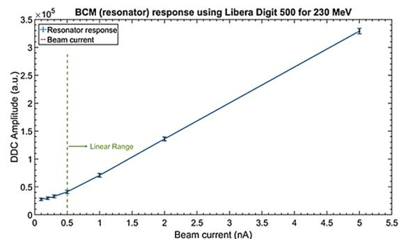
Figure 2: Prototype BCM response (in arbitrary units) measured by the customised Libera Digit 500. The beam current reference is measured using an IC.
