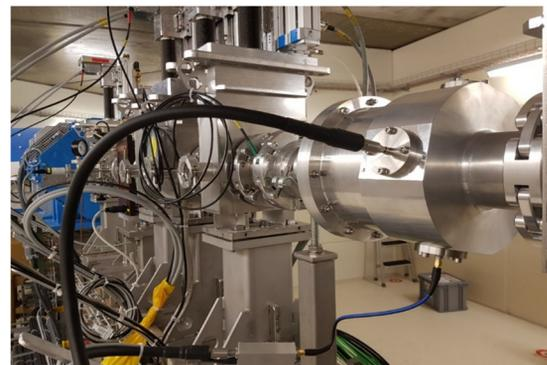
Figure 1: Prototype dielectric-filled re-entrant cavity resonator (BCM) installed at PROSCAN.
