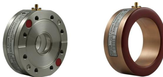
Figure 3: AWA uses two types of ICTs. In-flange (left) and In-air (right). The ceramic break is integrated into the in-flange model.
