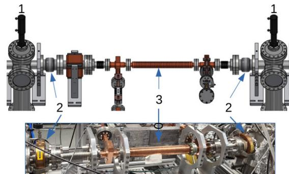
Figure 1: Experiment layout: Top: PETS vacuum installation drawing, Bottom: an installation photo illustrating the X-band PETS at AWA with some important diagnostics. Total distance from YAG to YAG is 144.5 cm. 1) YAG station 2) top: ceramic break for ICT 2) bottom: ICT as installed over ceramic break 3) PETS
