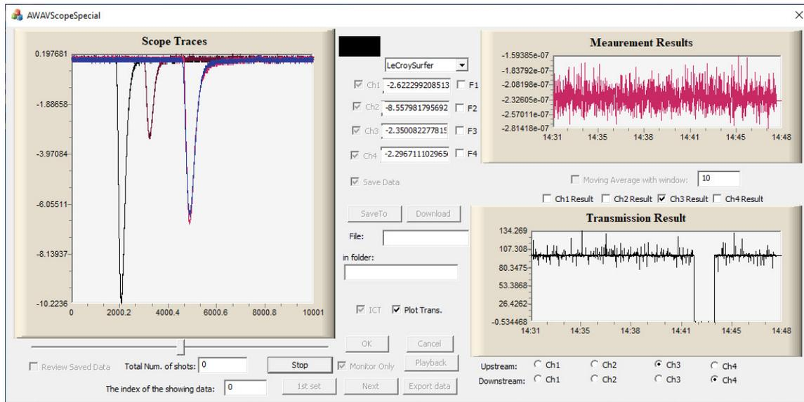
Figure 4: Screenshot of the ICT Monitor GUI during a recent experiment. Four ICT signals are being monitored along the beam line. The average transmitted charge is 245 nC, average transmission 100%.
