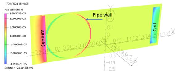
Figure 10: Eddy currents on the injection-beam-pipe.
