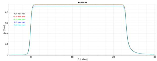
Figure 5: The B-field in the injected beam region.
