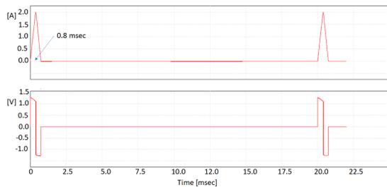
Figure 4: Consecutive pulses to excite the magnet at 1 Hz.
