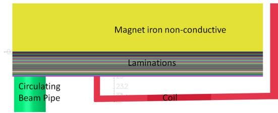
Figure 7: View of the 30 laminations, of 0.35 mm thick each.
