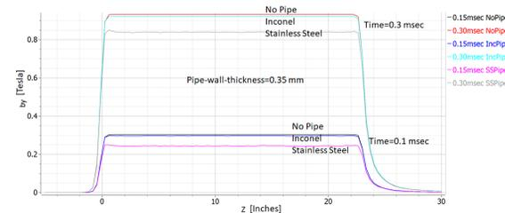
Figure 11: B-field of various material of the pipe at 625 Hz.
