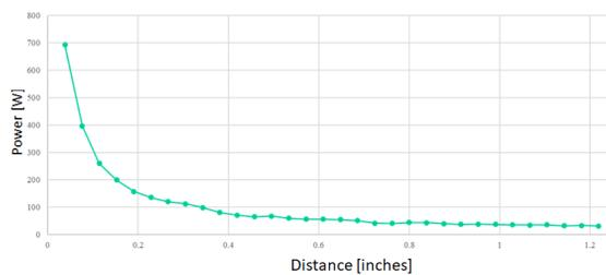
Figure 9: The power dissipation in each lamination.
