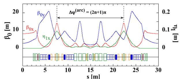
Figure 1: The optics and magnet arrangement of a unit cell. The squares shown at the bottom of the figure represent bending (blue), quadrupole (green), sextupole (orange) and octupole (red) magnets. Blue filled squares are bending magnets of the combined-function type.
