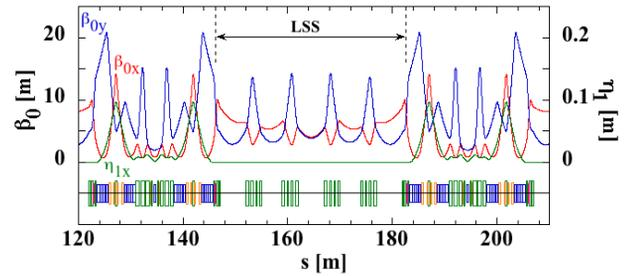
Figure 2: An example of the optics and magnet arrangement of a long straight section.
