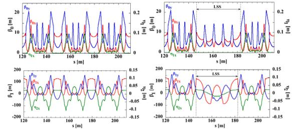
Figure 3: Matching of on- and off-momentum optical functions at the LSS. The energy-independent part  $(\beta_{0x}, \beta_{0y}$  and  $\eta_{1x}$ : upper) and the first-order energy dependence  $(\beta_{1x}, \beta_{1y}, \eta_{2x}$ : lower) are shown before (left) and after (right) inserting the LSS.
