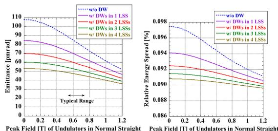
Figure 4: The emittance (left) and the relative energy spread (right) as a function of the undulator peak field. The dashed curve is for a bare ring without DW. The solid curves are for the ring with DWs and four curves are shown depending on the number of LSS used.
