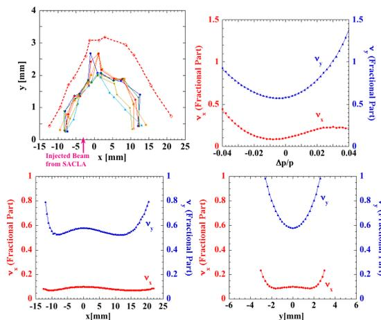
Figure 6: The DA observed at the injection point with  $\beta_{0x} = 20.0\text{ m}$  and  $\beta_{0y} = 2.3\text{ m}$  (left-upper), chromaticity (right-upper) and ADTS (bottom). In the figure of DA, the dashed line is for the ideal ring and the solid lines are for the ring with sextupole misalignment (rms  $25\text{ }\mu\text{m}$ , max.  $\pm 50\text{ }\mu\text{m}$ ).
