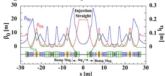
Figure 5: A tentative design of the injection cell.
