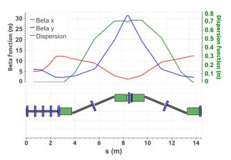
Figure 4: Variation of the optical  $\beta$ -function along the chicane.
