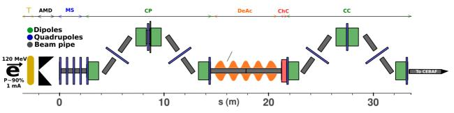
Figure 1: Conceptual layout of the positron injector for CEBAF.
