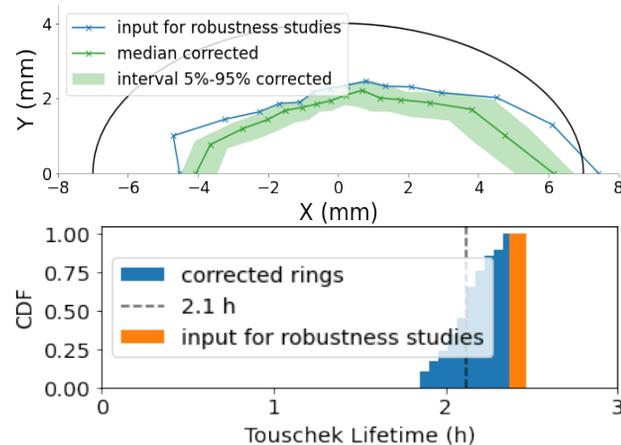
Figure 3: (TOP) DA and (BOTTOM) lifetime of the simulated machines, and the TDR as input for robustness studies.
