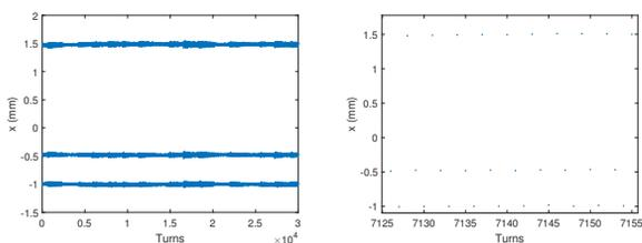
Figure 4: Turn-by-turn BPM data for horizontal plane. A bunch is excited to TRIB with the BxB kicker.
