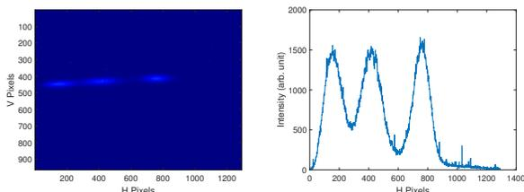
Figure 3: Pinhole camera image (left plot) and projection on the horizontal axis (right plot). A bunch is excited to TRIBs with the BxB kicker.
