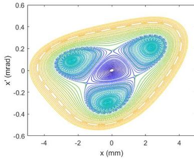
Figure 6: Contours on the  $x-x'$  phase space at the BxB kicker position. Lattice : TRIBs mode.
