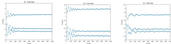
Figure 9: Centroid motion for varied K1 strength: 0.30 mrad (left plot), 0.44 mrad (middle plot), and 0.50 mrad (right plot). Results of particle tracking simulation with 2000 particles.
