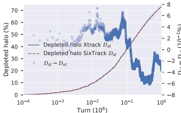
Figure 2: Halo depletion in HL-LHC with HEL in random pulsing in Xtrack (blue line) and SixTrack (red line). The blue dots represent the absolute difference between the two. Identical pulsing pattern, initial distribution, optics and normalized collimator settings were used.
