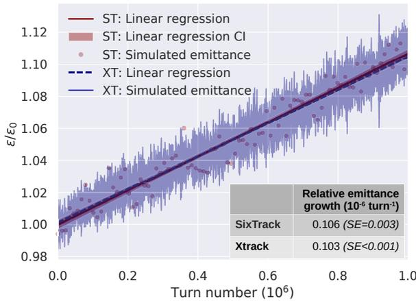
Figure 3: Simulated relative core-beam emittance growth  $\epsilon/\epsilon_0$  in SixTrack (ST) and XTrack (XT) assuming an uncompensated residual dipolar kick of 1 nrad at the HEL. The core-beam emittance growth estimated via a linear regression agrees within one standard error (SE).
