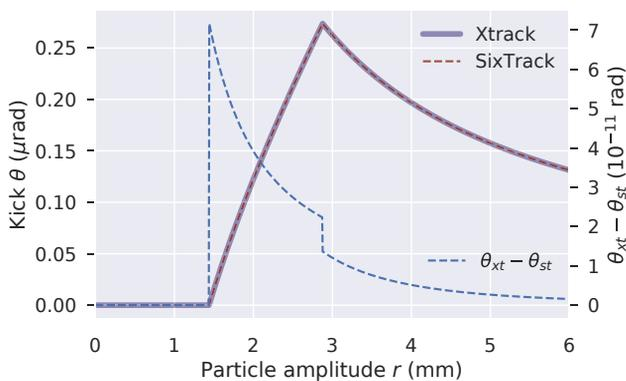
Figure 1: Kick  $\theta$  received by 7 TeV protons moving through a Hollow Electron Lens of 3 m length with 10 keV electrons, at 5 A current and inner and outer  $e$ -beam radii of  $r_1 = 1.44$  mm and  $r_2 = 2.88$  mm as calculated with Xtrack (blue) and SixTrack (red). The difference between the two results is visible on the right axis.
