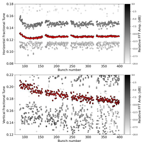
Figure 2: Horizontal (top) and vertical (bottom) bunch-by-bunch tunes measured through LHC BPMs in the SPS for an intensity of  $0.8 \times 10^{11}$  p/b.
