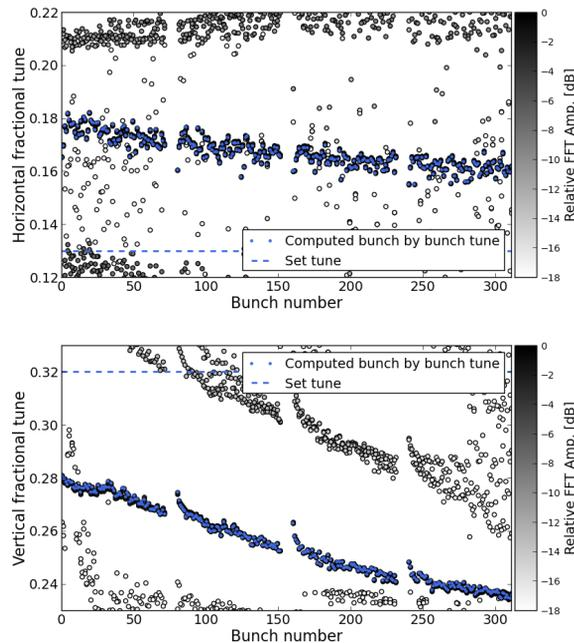
Figure 5: Bunch-by-bunch tunes obtained with PyHEADTAIL simulations, for high intensity of  $2.0 \times 10^{11}$  p/b.
