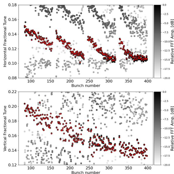
Figure 3: Horizontal (top) and vertical (bottom) bunch-by-bunch tunes measured through LHC BPMs in the SPS for an intensity of  $2.0 \times 10^{11}$  p/b.
