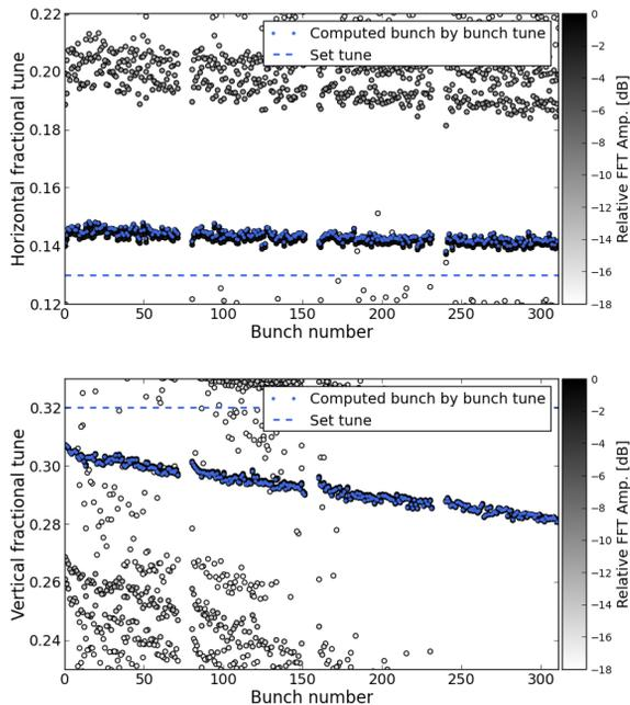
Figure 4: Bunch-by-bunch tunes obtained with PyHEADTAIL simulations, for low intensity of  $0.8 \times 10^{11}$  p/b.
