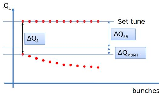
Figure 1: Schematic view of transverse tune shift along the bunch train (explanation in the text).
