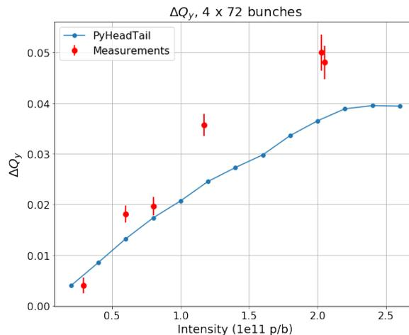
Figure 6: Tune shift of the fourth train with respect to the first train comparing measurements with simulations.
