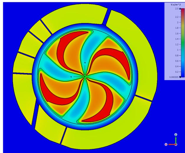
Figure 3: Magnet flux distribution of 230 MeV cyclotron.
