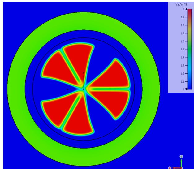
Figure 2: Magnet flux distribution of RC3/6.
