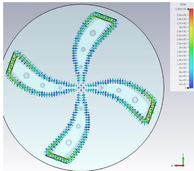
Figure 4: RF system of 230 MeV cyclotron in Push-Pull mode.
