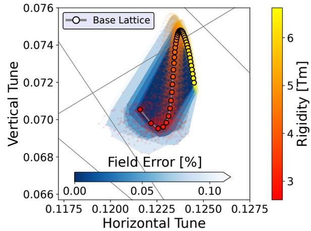
Figure 3: Cell tunes, with field errors up to  $\sigma(B) = 0.1\%$  applied separately to all multipoles. The footprint is the convex hull of the tunes calculated for 25 random multipole settings, set using a normal distribution truncated at  $\pm 3\sigma$ . Potentially destructive resonances are also shown.
