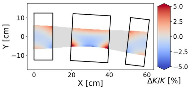
Figure 2: Fluctuations in focusing strength along the mid-plane closed orbits, for all rigidities. Tracking begins at the ‘F’ magnet centre. Outlines give magnet boundaries, with arbitrary aperture. Axes are ‘global’ top-down coordinates.
