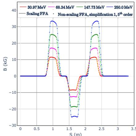
Figure 5: Magnetic field along the particle trajectory at different energies in a cell composed of scaling FFA elements and a cell with magnets whose magnetic field is truncated at the 5<sup>th</sup> order.
