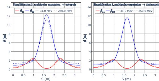
Figure 6: Horizontal and vertical  $\beta$ -functions (respectively  $\beta_{11}$  and  $\beta_{22}$ ) for different energies obtained for the third simplification and a multipolar expansion truncated at the 3<sup>rd</sup> or 5<sup>th</sup> order.
