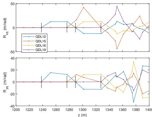
Figure 1: Calculated quadrupole-to-BPM trajectory response matrix for the QDL12 group. Top: horizontal; bottom: vertical.
