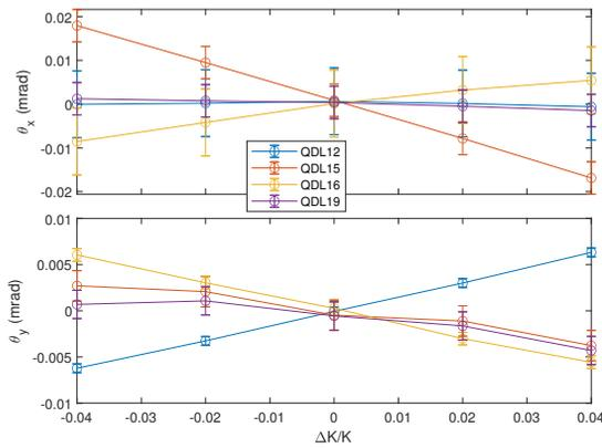
Figure 3: The kick angles derived from the induced orbit shifts for the QDL12 group example. Top: horizontal; bottom: vertical.
