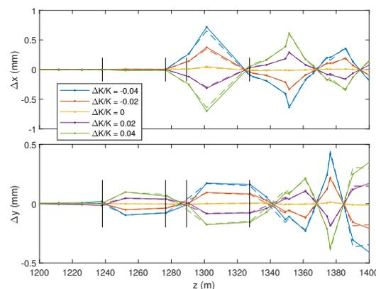
Figure 2: An example of measured induced orbit shifts for the QDL12 group. Solid lines are measured; dashed lines are calculated with the kick angles and the response matrix. Top: horizontal; bottom: vertical.
