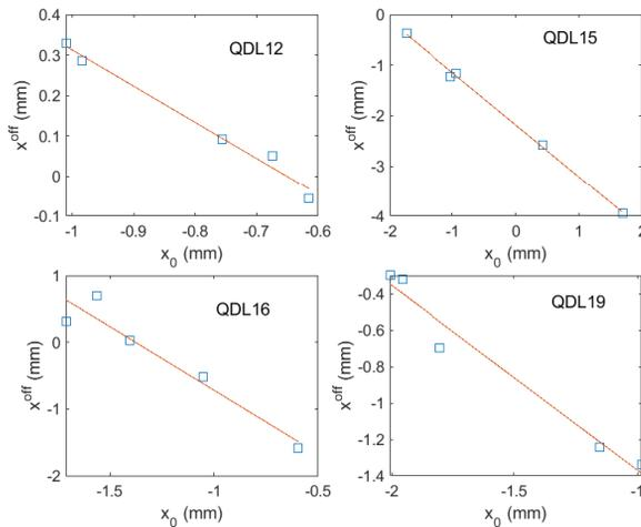
Figure 4: Horizontal quadrupole offsets vs. beam trajectory at the magnets for the QDL12 group. The quadrupole center corresponds to the zero crossing position.
