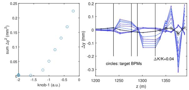
Figure 5: Minimization of the induced orbit shift for the vertical plane for the QDL12 group using a combined knob. Left: objective function vs. knob; right: the induced orbit shifts. The black curve corresponds to the minimal induced orbit.
