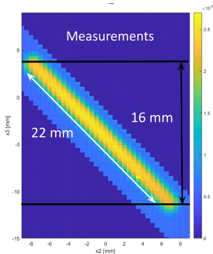
Figure 1: Measured gas jet profile on BGCv3 at CERN.
