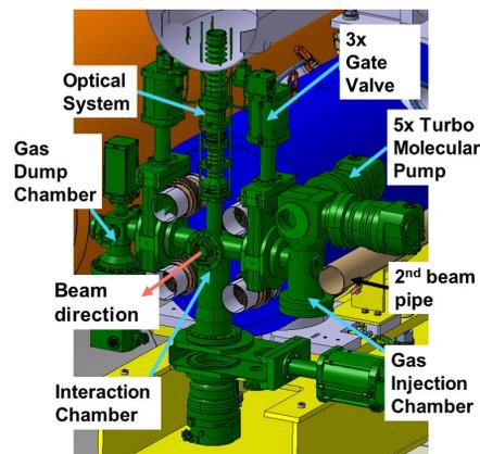
Figure 4: 3D model BGCv4 integrated in the HEL.
