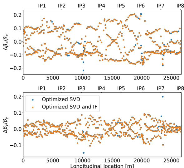
Figure 1:  $\beta$ -beating computed with and without IF-cleaning.
