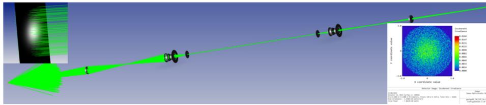
Figure 1: The full 3 stage optical system simulated in Zemax Optic studio in non sequential ray tracing mode.
