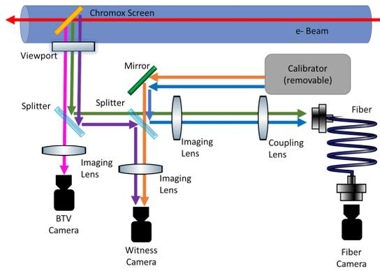
Figure 3: Sketched layout of the experimental setup installed at CLEAR showing the fiber installation with its calibration line in parallel to the operational BTV.
