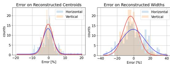
Figure 5: Errors distributions for the estimated beam centroid and width with the Pix2Pix trained on beam data.
