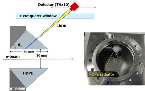
Figure 3: HDPE radiator shape and detection apparatus for ChDR (upper), and a view of assembly on the beam line in the vacuum chamber (lower).
