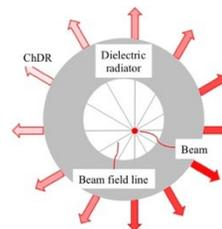
Figure 1: Cross section view of cylindrical hollow radiator and ChDR.
