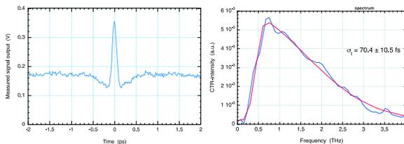
Figure 2: An interferogram of TR measured by a Michelson interferometer (left), and frequency spectrum (right).
