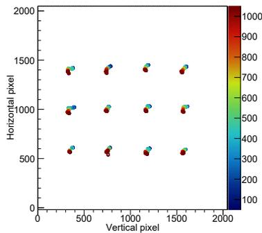
Figure 5: Pinhole image peaks measured at the beam current ranging from 50 mA to 1050 mA in LER.
