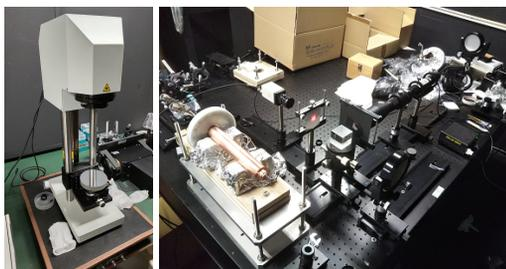
Figure 2: Interferometers used for quality assurance testing. Left: Fizeau interferometers Olympus KIF-201. Right: Interferometer setup using a He-Ne laser.
