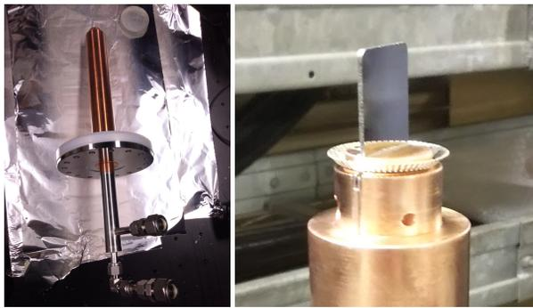
Figure 1: Left: The mirror holder consisting of a water-cooled split cylinder of copper. Right: Mirror mounted in water-cooled copper holder.
