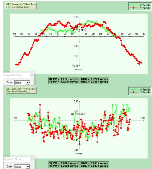
Figure 3: The mirror surface flatness. Top: the result obtained in the first test. Bottom: the result obtained in the second test.
