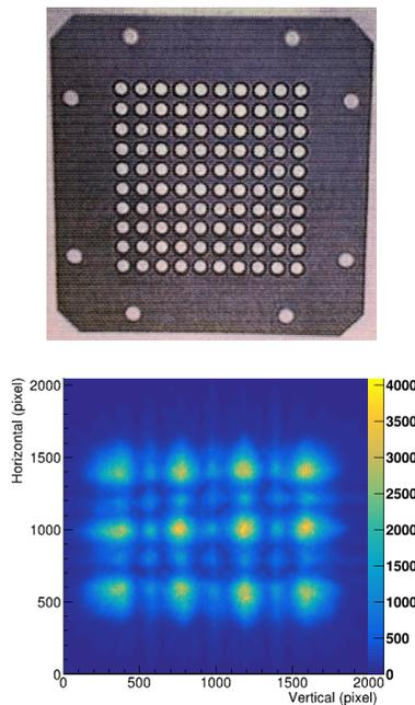
Figure 4: Top: A square array screen. Bottom: Measurement for Hartmann spots produced by the square array screen.
