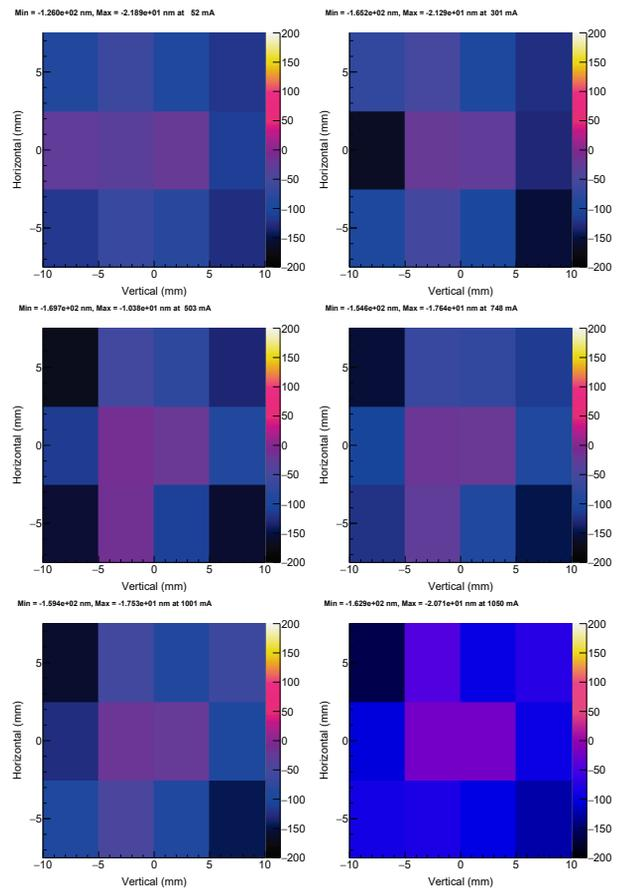
Figure 6: Mirror surface deformation in LER at the beam current ranging from 50 mA (top left), 300 mA (top right), 500 mA (middle left), 750 mA (middle right), 1000 mA (bottom left), and 1050 mA (bottom right).
