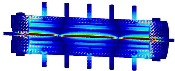
Figure 7: An eigenmode simulation of the Brockhouse beam-line wiggler performed using GDFIDL [6] at 219 MHz.
