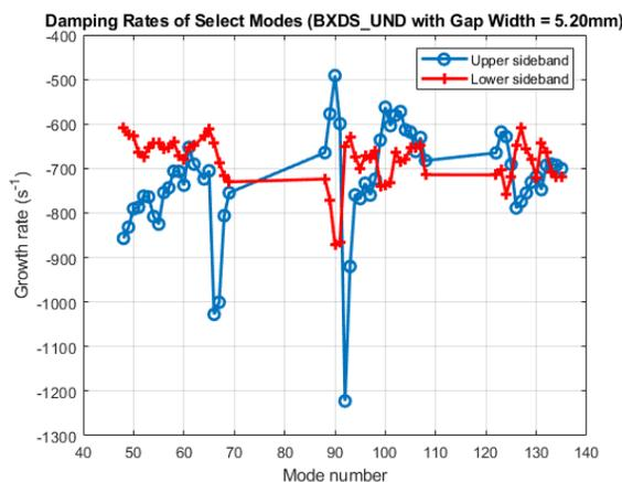
Figure 2: Selection of modal damping rates for the In-vacuum Undulator on the Brockhouse beamline (BXDS\_UND).
