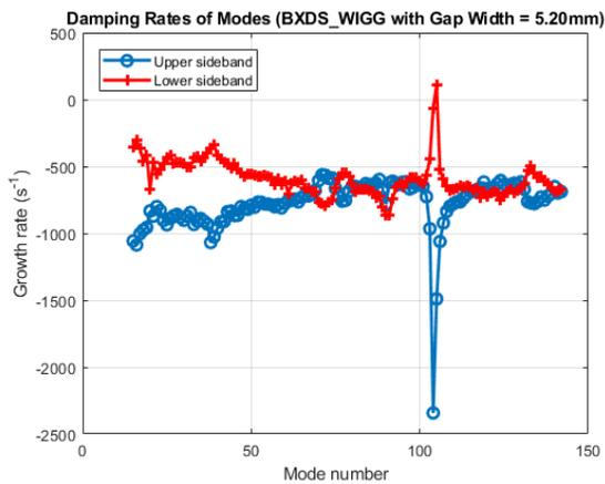
Figure 5: Decay rates on the Brockhouse Wiggler at the minimum gap width of 5.20 mm. Note the large spike in the growth rates present around mode 105 (corresponding to mode 180 on the lower sideband).
