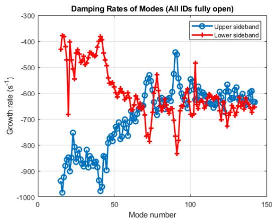
Figure 1: Structure of modal damping rates. Note that the upper and lower sidebands are the sidebands of the revolution harmonic, and correspond to the lower and upper halves of the 255 scanned modes, respectively. The top and bottom 15 modes are omitted.
