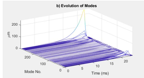
Figure 3: Typical result from a grow/damp measurement at the CLS storage ring. Mode damping was suspended for 23ms. The excitation of the highest and lowest modes are believed to be caused by the resistive-wall effect.
