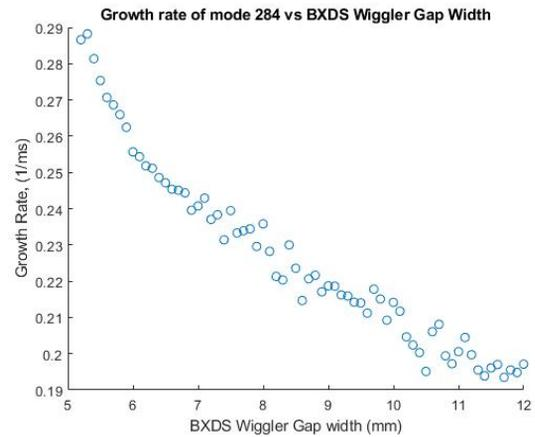
Figure 4: Modal growth rates of the top 284th mode. The growth rate slows as the gap width increases.
