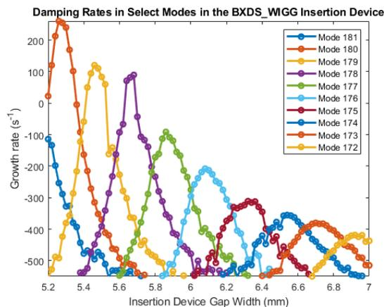
Figure 6: Decay rates of modes around mode 180. Each subsequent mode has a peak instability at a different gap width. Data on each peak is found in Table 1.
