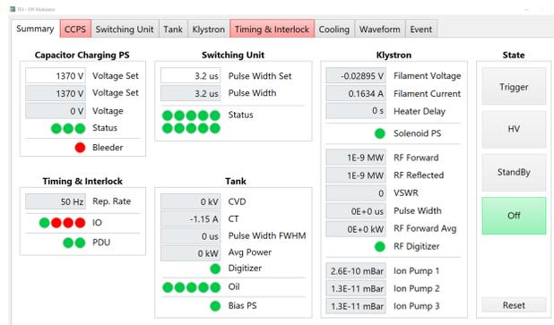
Figure 5: RF Modulator interfaces.
