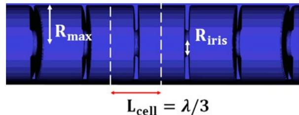
Figure 1: DLWG cavity array.
