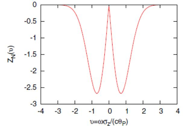
FIG. 3. Imaginary part of normalized cross impedance, where  $v = \omega \sigma_z / (c \theta_p)$ .
