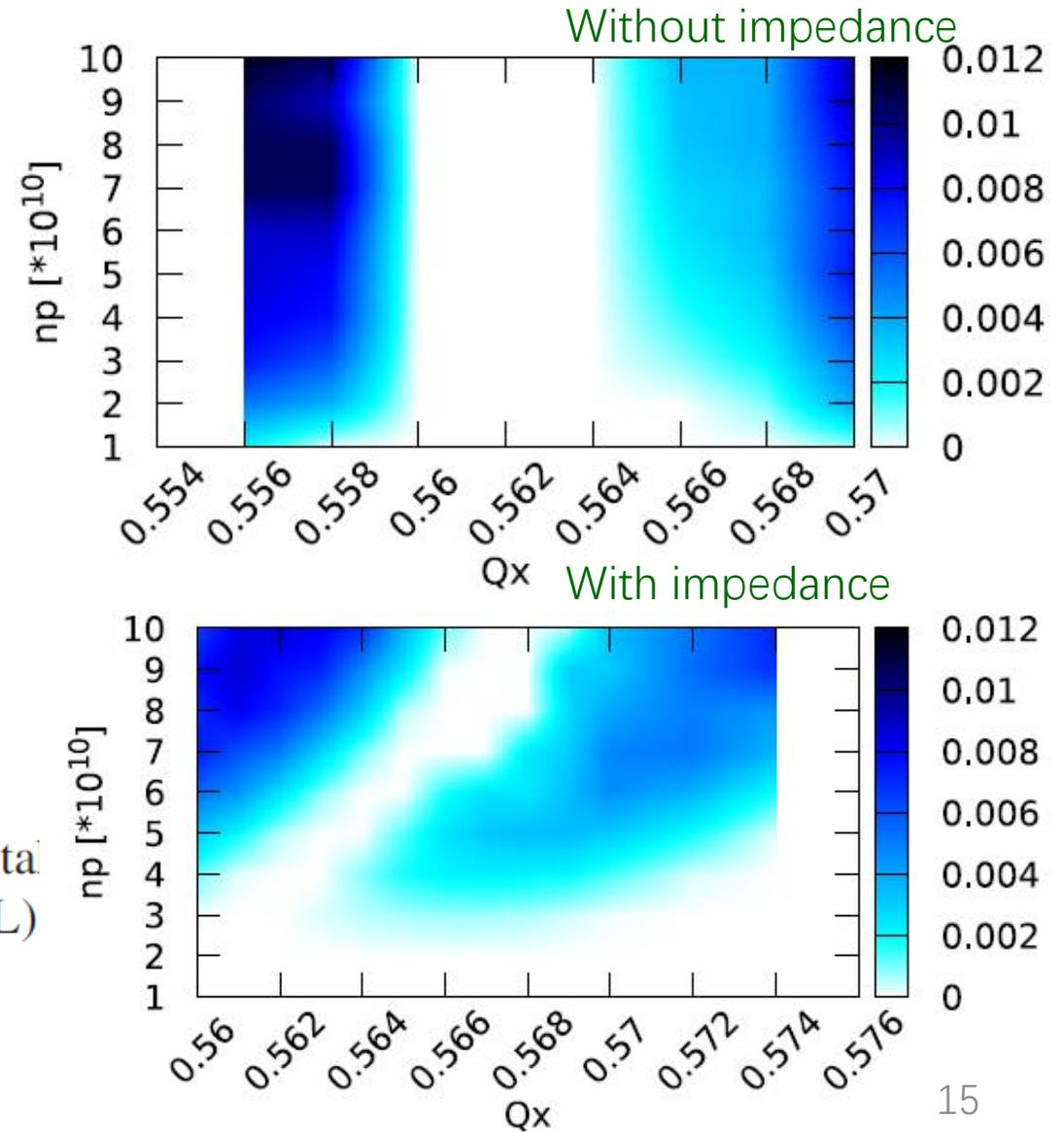
FIG. 3. The horizontal beam size growth rate versus horizontal tune with and without longitudinal coupling impedance (ZL) Beamstrahlung (BS) effect is turned on.
