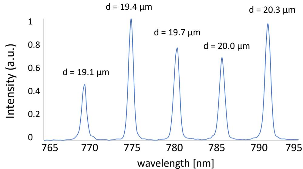
Second harmonic parameters (25°C,  $d = 19.4 \mu\text{m}$ )
