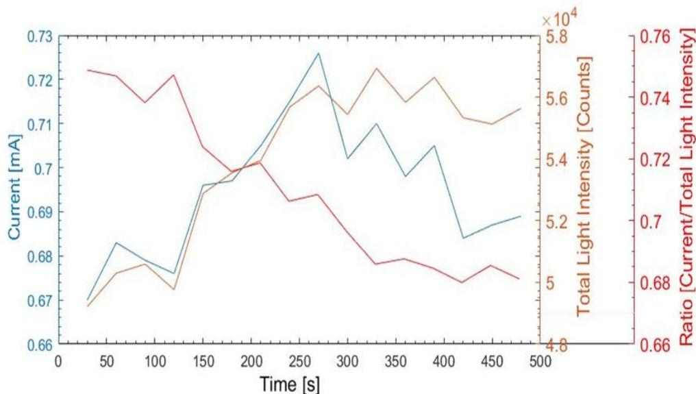
“Total light intensity” is the light intensity at every measured wavelength summed together. These results did give a clear relationship between the light intensity and current measured with respect to time. As the current fluctuated the light intensity appeared to follow the same changes in terms of increasing and decreasing by similar proportions.
