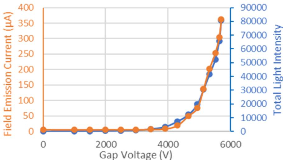
Looking for light emission correlation with the Fowler Nordheim Theorem. Light intensity when plotted with respect to voltage gives a plot that resembles the emission plot.
