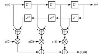
Figure 3-24: Hilbert Transformer Pipeline structure
