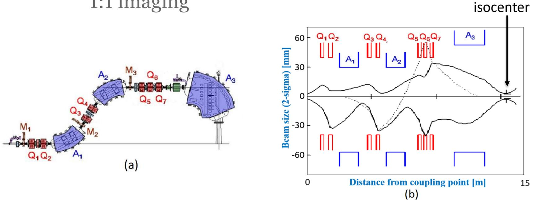
Figure 1 : (a) Shows the PSI's Gantry 2 layout, with three dipoles (elements A) and seven quadrupoles (elements Q). (b) Shows the 2-sigma beam envelope and the dispersion (dashed line,  $dp/p=0.7\%$ ) along the gantry with 1:1 imaging (The lower half shows beam envelope in X-plane (bending plane) and the upper half shows envelope in Y-plane.)
