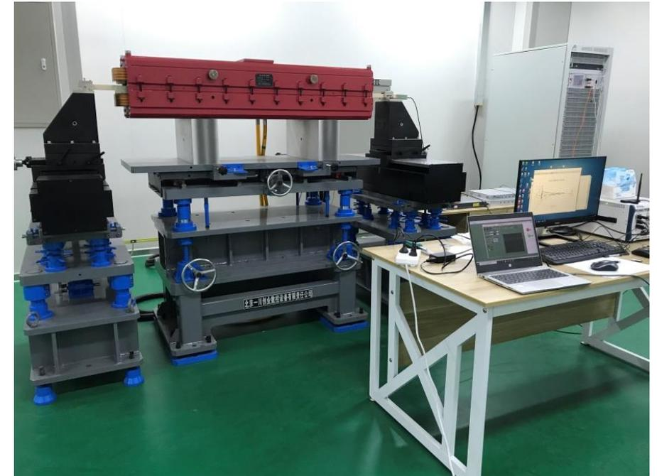
The magnetic measuring system consists of a over 2.0m long measuring coil, a mechanical platform with a stroke within plus or minus 300mm, a motion control system and a signal acquisition equipment.
