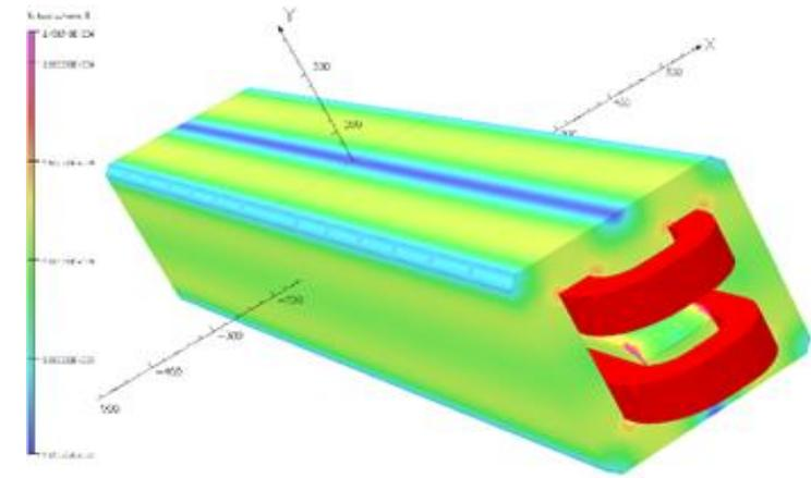
Fig. 1 Physical Design Model of Dipole Magnet for HEPS Booster ( HEPS-BS-34B )
