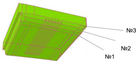
Fig. 5. Quarter pole chamfered dipole.
