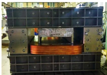
Fig. 4. Appearance of the assembled CR dipole magnet.
