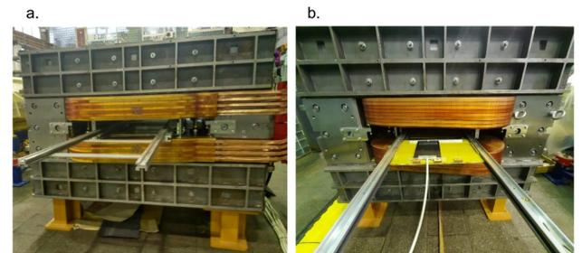
Fig. 7. a, b - CR dipole precision measurement system based on carriage with Hall sensors, plate and rail
