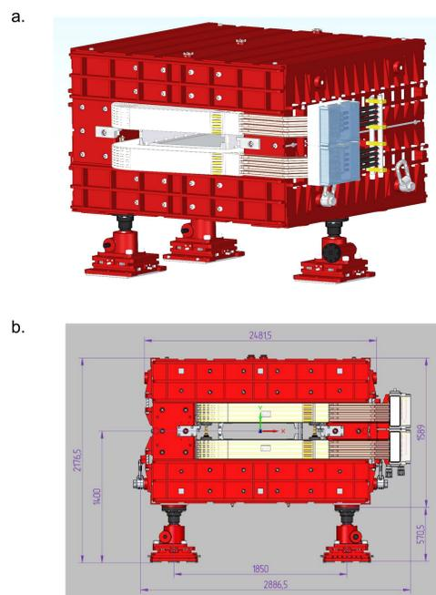
Fig. 3. a, b - 3D model of a dipole magnet CR
