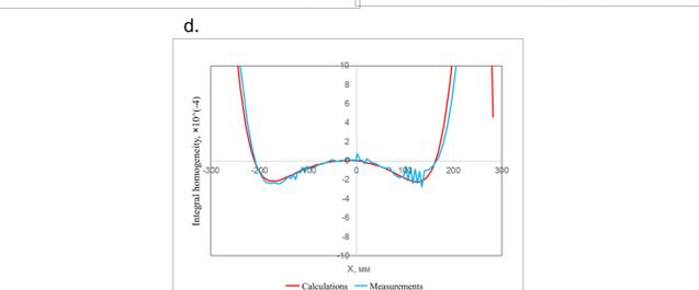
Fig. 9. A plot of the integral homogeneity at  $I = 750$  A: a. no gradient deduction (calculations, no chamfer and final); b. with the deduction of the gradient (calculation and version without chamfer); c. calculation and variant with chamfer № 1; d. calculation and variant with chamfers № 1 and № 3
