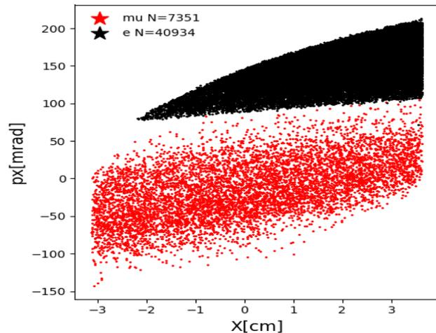
phase spaces of muons and the positrons are separated by ESD in baby scheme
