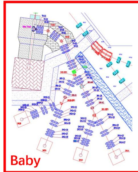
CSNS will build a muon source at the end of the RTBT. In the current design, the muon source propose two schemes, namely the **baseline scheme** and the **baby scheme**. High voltage electrostatic deflectors (ESD) are used to deflect the beam in the two schemes. A **three-channel ESD** with **400 kV HV** is employed in the baseline scheme and a **210 kV dual-channel ESD** in the simplified scheme.
