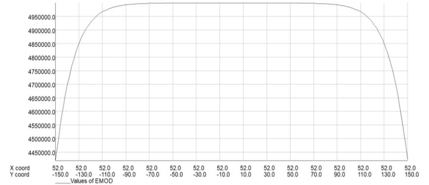
2D simulation:  $E_0=5\text{MV/m}$ ,  $E_{\text{max}}=5.76\text{MV/m}$ ,  $\beta = 1.15$
