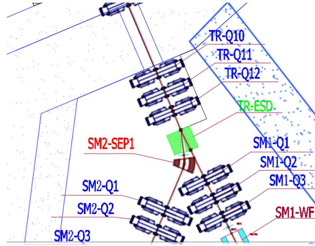
Combination of dual-channel ESD and septum magnet for baby scheme
