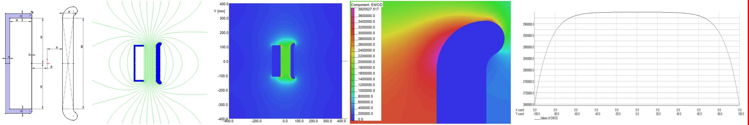
2D simulation:  $E_0=3\text{MV/m}$ ,  $E_{\text{max}}=3.92\text{MV/m}$ ,  $\beta = 1.31$
