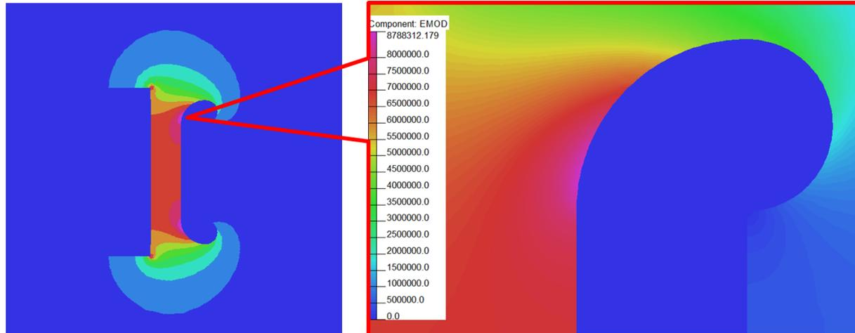
The maximum field intensity is concentrated at the end of the electrode. The larger the chamfer radius  $R_1$ , the smaller the maximum electric field intensity and the smaller the electric field concentration factor.
