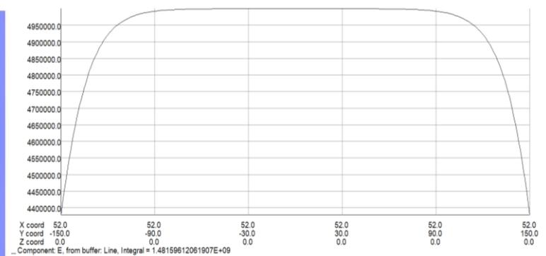
3D simulation:  $E_0=5\text{MV/m}$ ,  $E_{\text{max}}=6.58\text{MV/m}$ ,  $\beta = 1.32$
